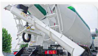
Extended discharge chute
